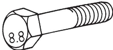
[Usually, material strength identification on bolt head is with number (i.e., 8.8, 10.9, etc.)]
