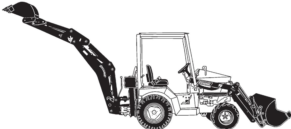
**This is the position machine must be in to check proper level in hydraulic tank.**
