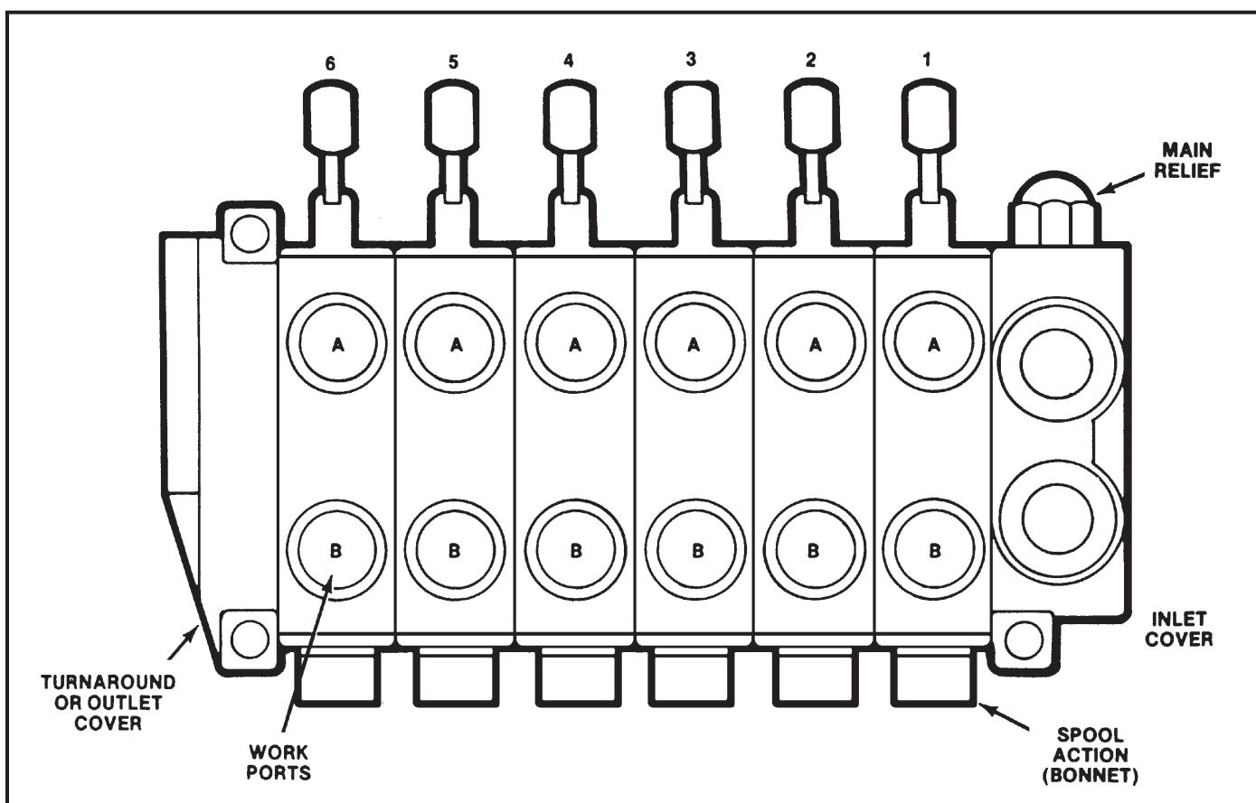
1. Before disassembly, it is suggested that each valve section be marked numerically to avoid incorrect reassembly.
